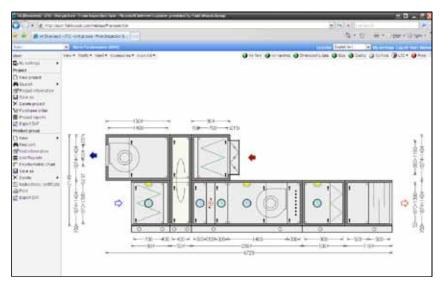
To ensure correct configuration of hygiene units, ACON has a Hygiene Verification Check function that helps the user to configure a unit compliant with VDI 6022 for standard hygiene or EN 1946-4 for hospital environments. ACON provides clear recommendations and instructions to ensure that the unit meets relevant standards. Fläkt Woods recommends that the user has good prior experience of hygiene projects, as certain standard requirements must be met by the electrical technician and the customer.
